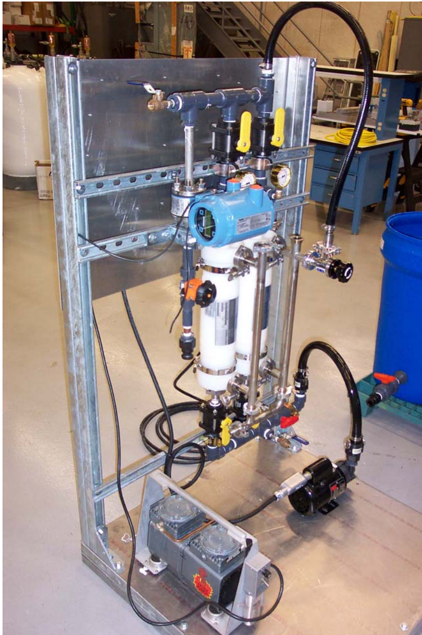
Figure 3. Gas Extraction test apparatus at LLNL. Membrane contactors are housed in white vertical cylinders; diaphragm pump sits on the floor.
